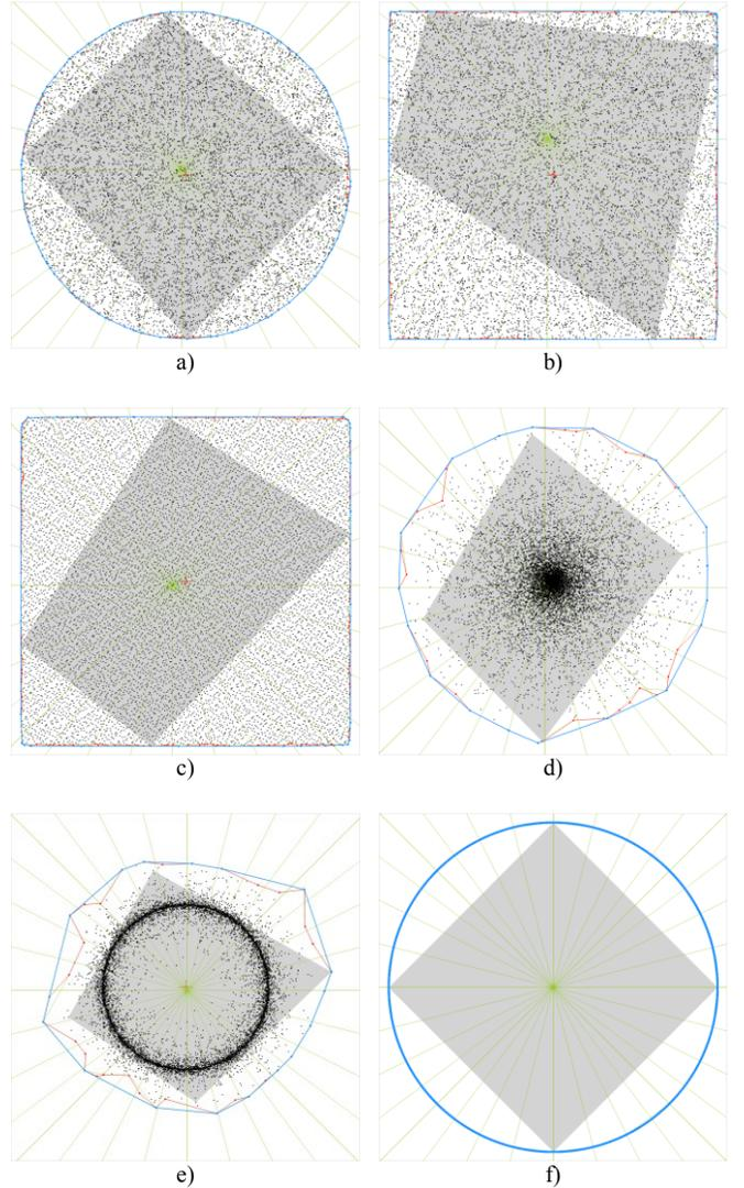
Fig. 8. Convex hulls of points with different distributions: a) uniform points in circle, b) uniform points in square, c) Halton points, d) Gauss points, e) Gauss Ring points and f) points on circle.
